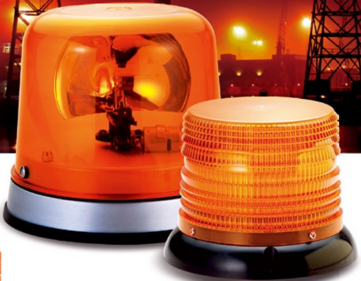
CAX76-LED/R Rotating LED beacon • 12-40V DC, 0.75A • 8 x 2W LEDs • Flash rate: 120/min.
