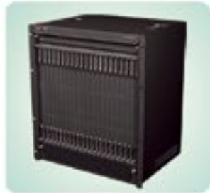
PE60S-series modular IP matrix • 512 inputs, 128 outputs • Extends up to 65, 535 channels • Built-in code converter • Compatible with Pelco D/P, Panasonic, Samsung, Vicon, Kalatel or OEM products • With SDK; compatible with future developments
